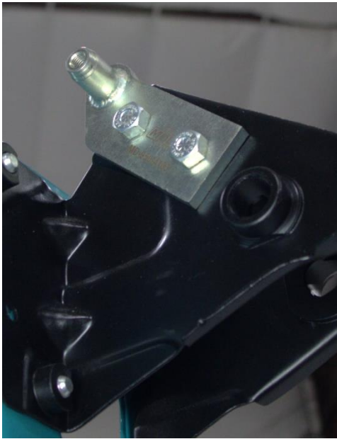
Left Picture: Bracket installed with MDL hardware for non-power brake cars.
